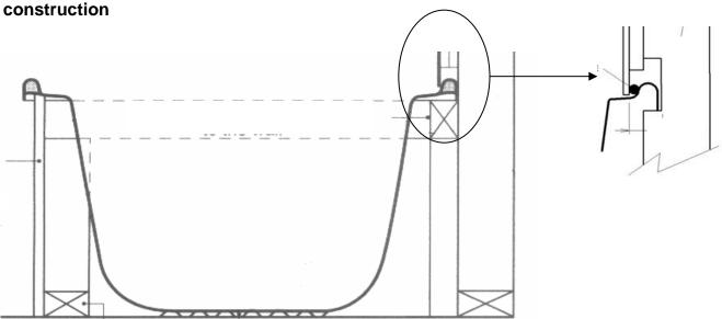
Bath must be fully supported at all times, it is **not** a self supporting bath. Failure to fully support bath will void warranty.
